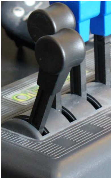
Throttle lever in detent / idle position
